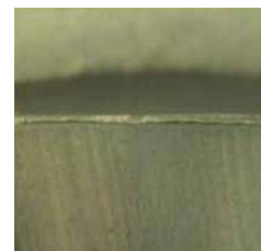
YG-1 X5070 (Total Milling Length : 540m)
